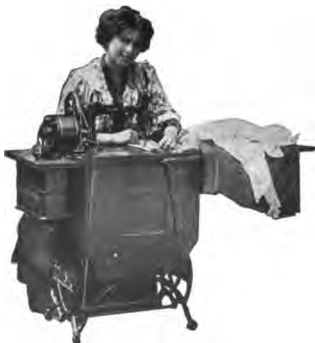
FIG. 105. — A motor runs the sewing machine.
